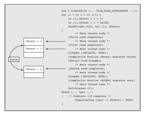
Figure 14-2 Asynchronous I/O with Completion Routines
