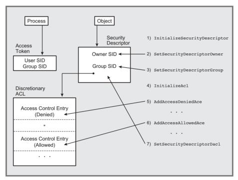
Figure 15–1 Constructing a Security Descriptor
