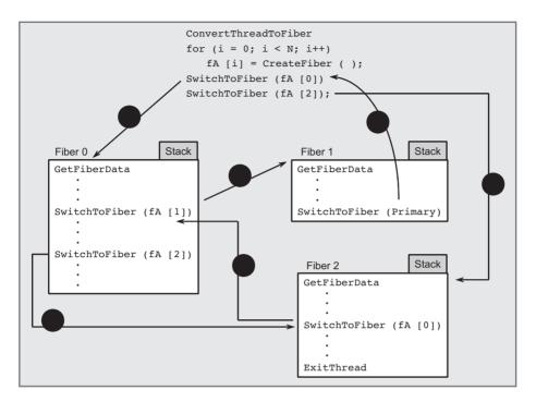
Figure 7–5 Control Flow among Fibers in a Thread
