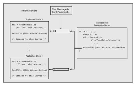
Figure 11-3 Clients Using a Mailslot to Locate a Server
