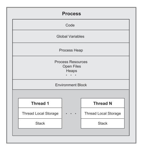
Figure 6–1 A Process and Its Threads
