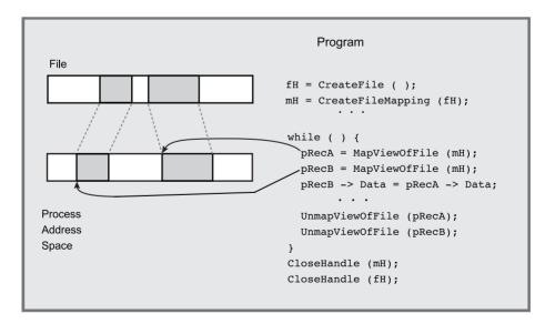
Figure 5–3 A File Mapped into Process Address Space
