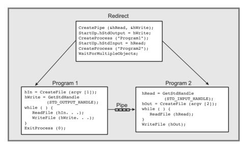
Figure 11-1 Process-to-Process Communication Using an Anonymous Pipe
