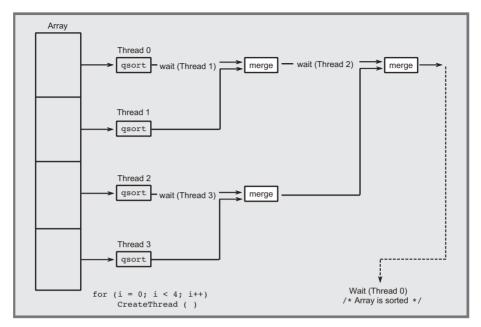
Figure 7–2 Merge-Sort with Multiple Threads
