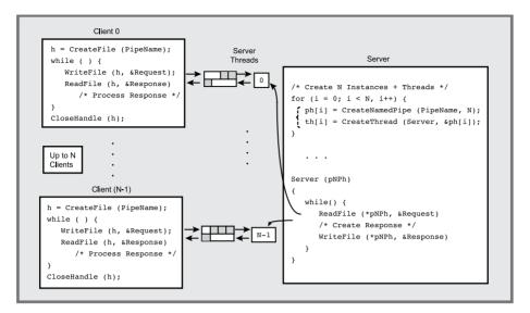
Figure 11-2 Clients and Servers Using Named Pipes
