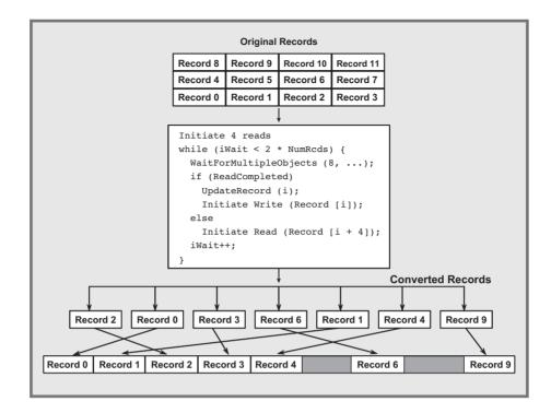
Figure 14–1 An Asynchronous File Update Model
